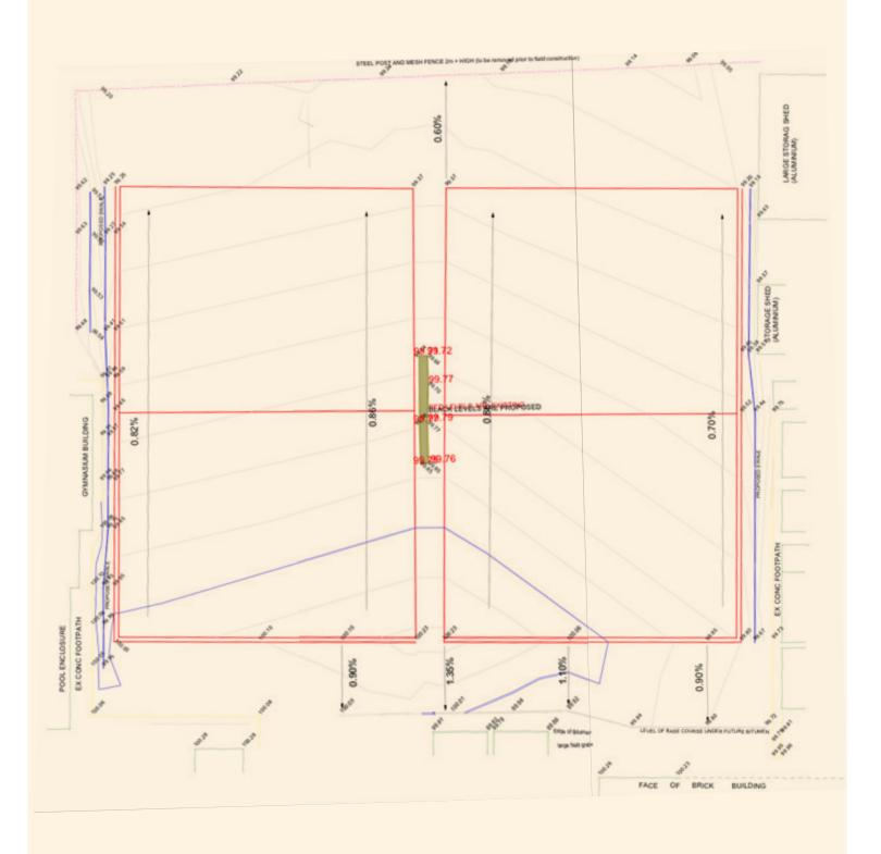
After surveying the field and calculating the soil available and imported turf sand the above design was engaged. As over 7,000 m3 of soil had to be moved, 2 dozers with machine control had been engaged to rough in the surface to +/-25mm with final trimming done with a tractor and laser box blade.
