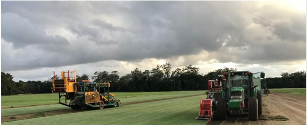
Turfing on the playing, turf was harvested razor thin to minimise any imported soil contamination as turf washing was not an option. The choice of using slabs was also preferred due to the capacity of harvesting slabs thinner than maxi rolls are able to be. Three turf harvesters had been used to harvest and install the turf in as short of a time as possible
